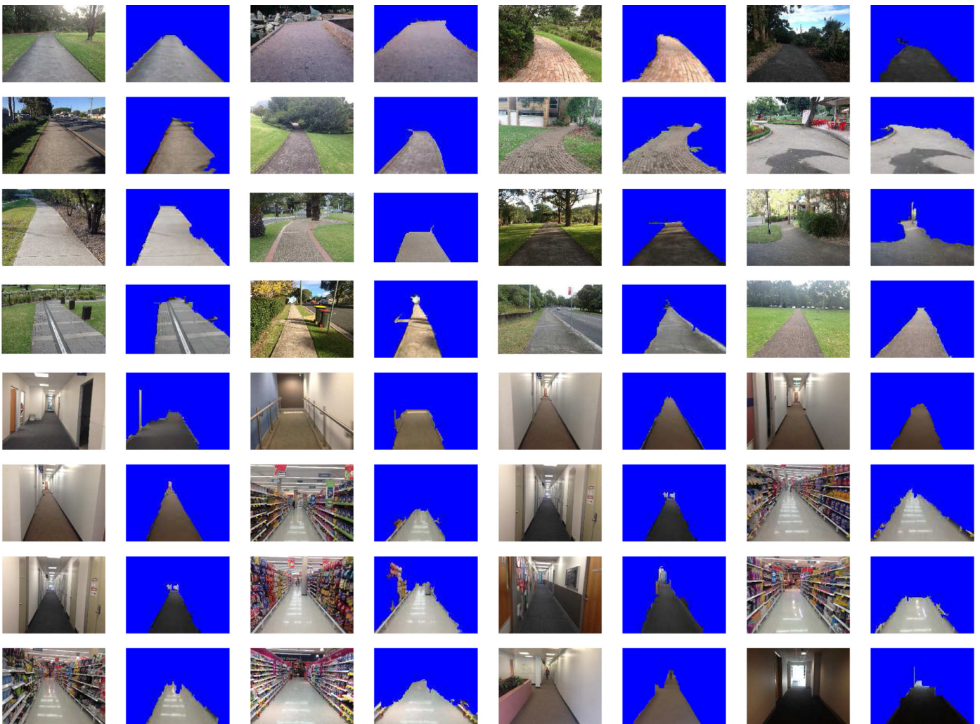
Fig. 8. Visual sample results of the proposed method for detecting pedestrian lanes in indoor and outdoor environments. Columns 1, 3, 5 and 7: input images. Columns 2, 4, 6 and 8: detected lanes. See the electronic color images. (For interpretation of the references to color in this figure legend, the reader is referred to the web version of this article.)
